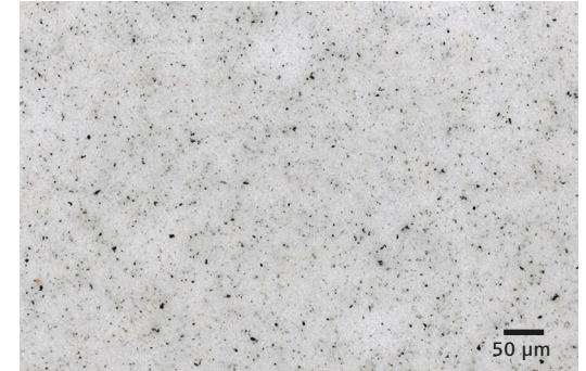
Particle analysis, brightfield, objective: EC Epiplan-NEOFLUAR 20×/0.5
